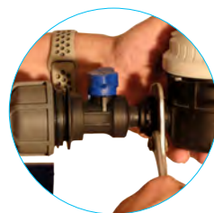
5. Tighten free nut on the water meter, using a wrench for the last 1/4 turn
